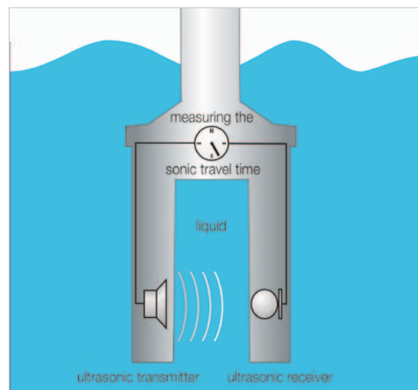
Measuring principle of sonic velocity
