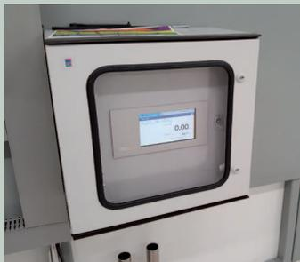
The first LiquiSonic® concentration analyzer was taken into operation at the new  $H_2SO_4$  plant in Harjavalta in August 2018 to measure sulphuric acid concentration 90...100 wt% at the outlet of the plant to storage tank.
