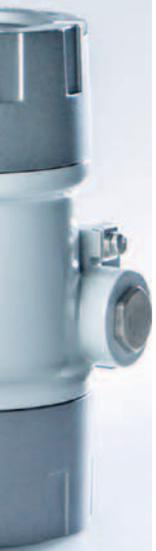
LiquiSonic® is an inline analytical system, that detects the concentration in a liquid directly in the process and without any time lag. The device is based on the accurate measurement of sonic velocity and temperature and enables so the monitoring of processes and complex reactions.
