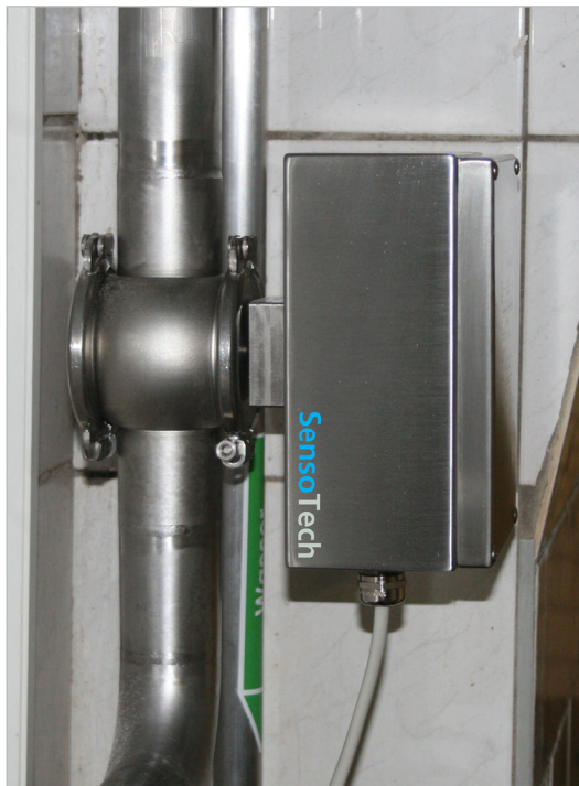
LiquiSonic® Plato application at the wort cooler
