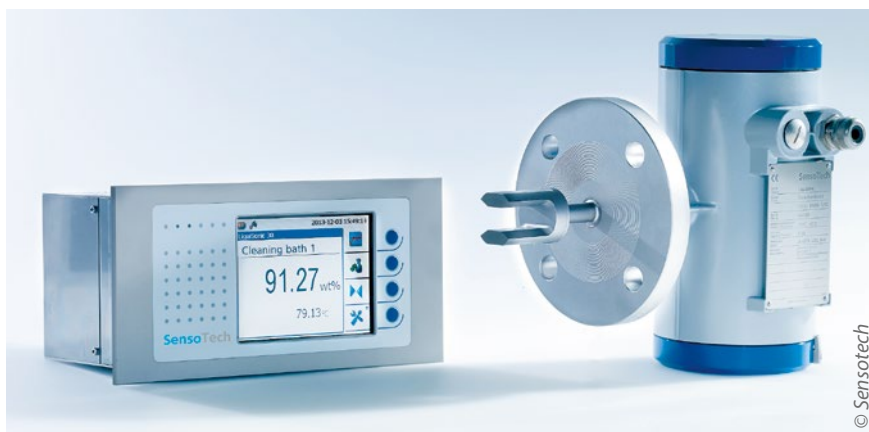
Figure 2: The measuring system monitors the concentration of the cleaning agent or the degree of contamination directly in the bath and makes the measured values available online.
