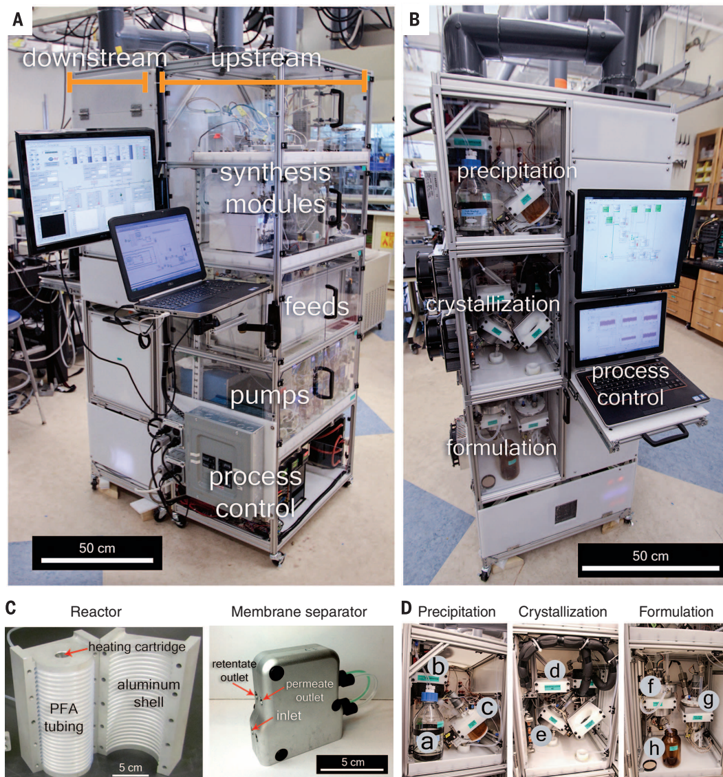
Fig. 1. Reconfigurable system for continuous production and formulation of APIs. (A)
