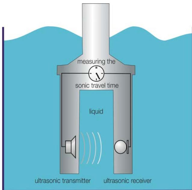
**Figure 1.** The measuring method of the LiquiSonic sensors is based on sonic velocity that is determined temperature-compensated by a run-time measurement and used to derive concentrations in liquids.
